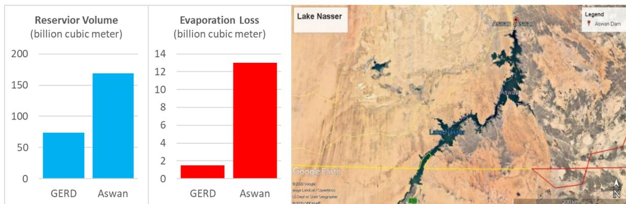
Figure 5: Reservoir size and water loss comparison between GERD and Aswan Dam
